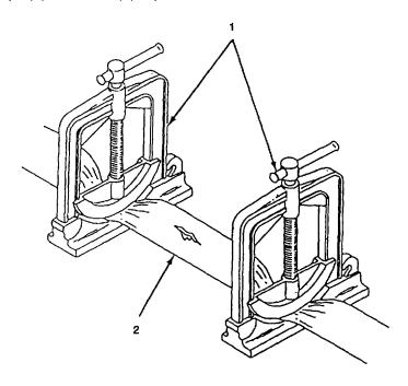
Figure 3-1. Installing Hose Clamps
