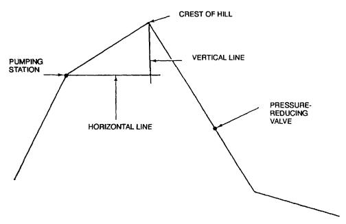
Figure 2-5. Pressure- Reducing Valve Location
