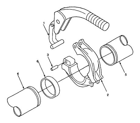
Figure 2-7. Boltless Coupling
