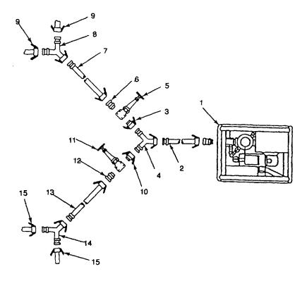
Figure 2-25. Hypochlorination Unit and First Wye-Connection
