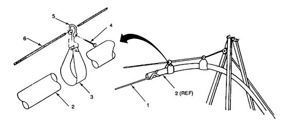
Figure 2-12. Installing Saddle on Hoseline
