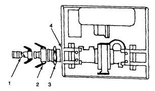
Figure 2-45. Discharge Hose Couplings and Hypochlorination Unit
