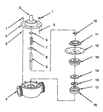
Figure 5-3. Main Valve Assembly
