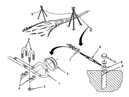
Figure 2-11. Wire Rope Loop
