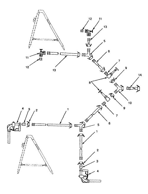
Figure 2-46. Disassemble Distribution Point
