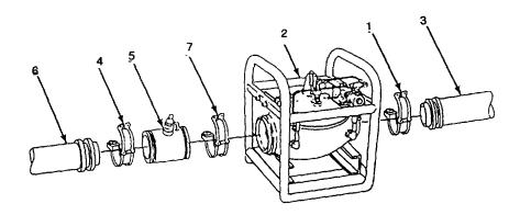
Figure 2-39. Disassemble Pressure-Reducing Valve
