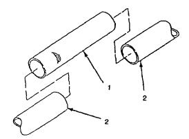
Figure 3-2. Removing Damaged Hose Section
