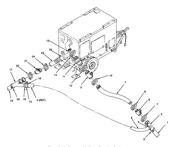
Figure 2-41. Disassemble Boost Pumping Station
