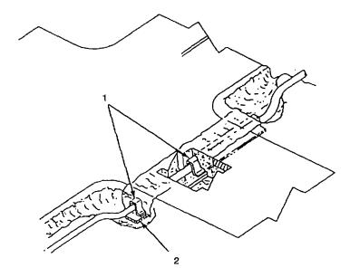
Figure 2-40. Disassemble Road Crossing Guard
