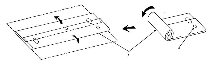
Figure 2-19. Proper Unroll and Unfold of Storage Tank
