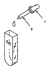
Figure 2-32. pH Test Cell
