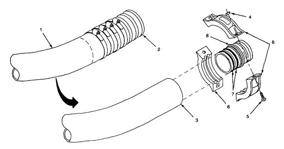
Figure 3-5. Female Hose Adapter Assembly
