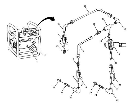
Figure 5-1. Pressure-Reducing Control
