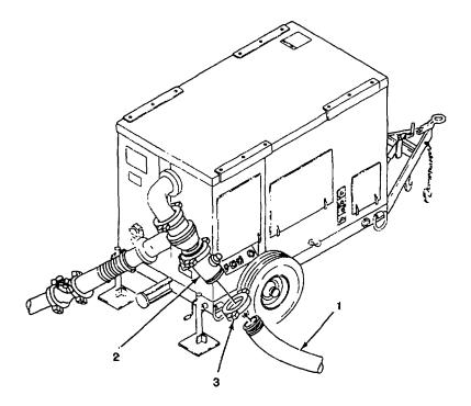
Figure 2-8. Connecting 10-MIIe Segment to Lead Pumping Station
