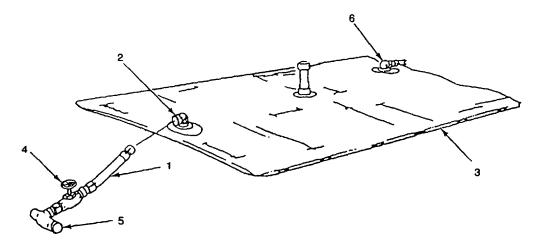
Figure 2-21. Connecting Discharge Hose Assembly
