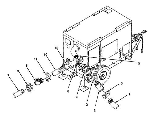
Figure 2-42. Disassemble Lead Pump Station
