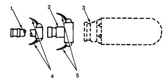
Figure 2-22. Tank, Reducer and Hose Assembly
