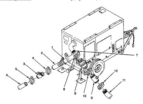
Figure 2-16. Lead Pumping Assembly
