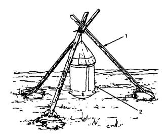
Figure 2-28. Potable Water Storage Bag
