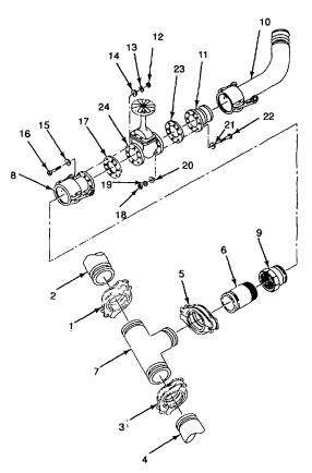
Figure 2-43. Disassemble Storage Assembly
