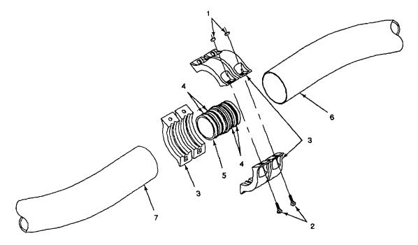
Figure 3-3. Mid-section Hose Adapter Assembly
