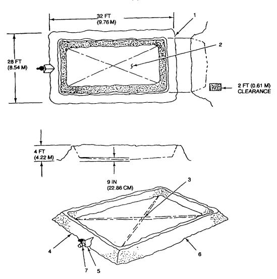
Figure 2-18. Storage Tank Location Preparation
