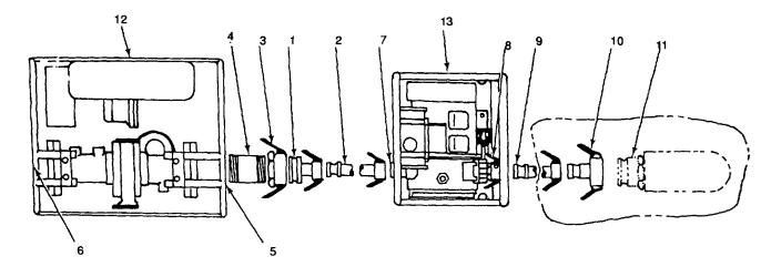
Figure 2-47. Hypochlorination Unit, 125 GPM Pump, and Storage Tank Assemblies
