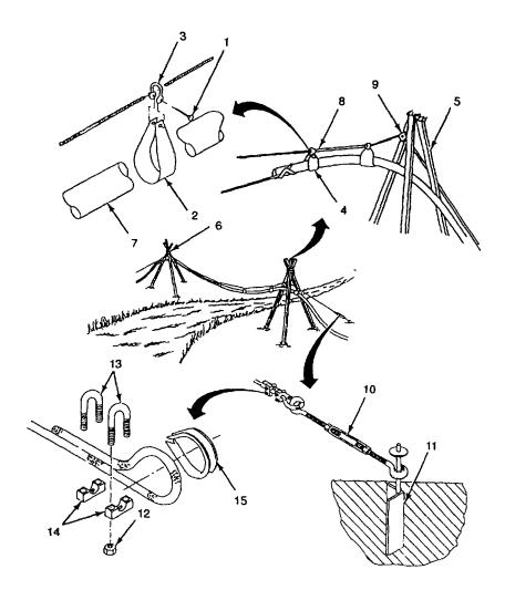
Figure 2-38. Disassembly of Suspension Device
