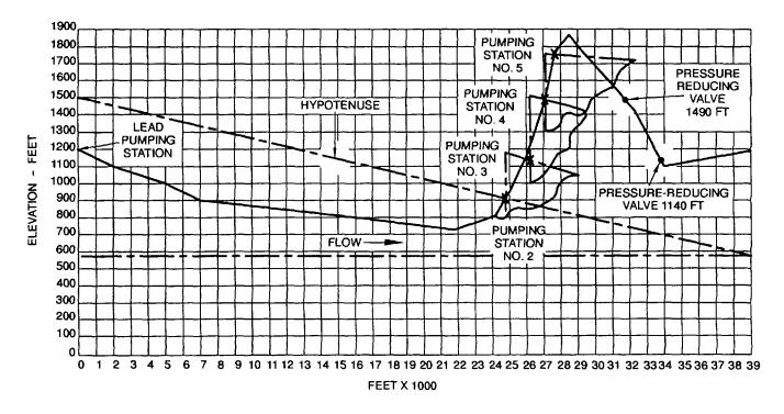
Figure 2-4. Ground Profile and Pump Spacing Triangle
